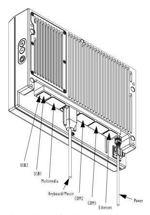
Figure 1.3 Back Of 8560: Ports And Safety Label
