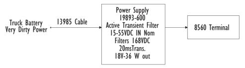
Figure 4.13 Connection Method for Active Transient Filter Power Supply
