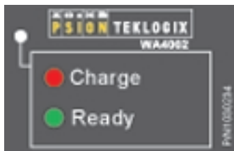
Figure 8.11 Battery Charge Status
