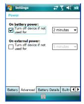
The Advanced tab allows you to manage battery consumption.
