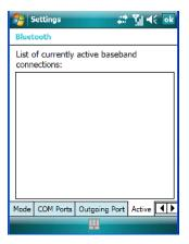
This tab displays the currently active *Bluetooth* connections, listing the device name(s). The type of link is also included with the device name(s). Keep in mind that the information listed in this tab is 'view only'; it cannot be edited.
