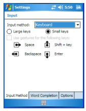
This screen is displayed when you choose *Keyboard* in the *Input method* drop-down menu. You can use it to customize the soft keyboard. You can choose *Large Keys* or *Small Keys* to increase or decrease the size of the keys displayed on the soft keyboard.
