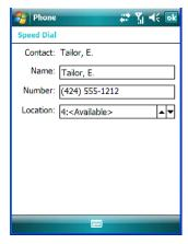
A sequential speed dial key is automatically assigned in the *Location* field. You can tap on the *Location* dropdown menu and change the auto assignment.
