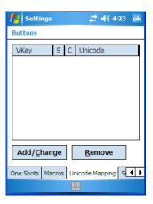
The *Unicode Mapping* tab is used to map combinations of virtual key values and [CTRL] and [SHIFT] states to Unicode<sup>TM</sup> values. This tab shows the configured Unicode character along with the Unicode value. For example, "a (U+0061)" indicates that the character "a" is represented by the Unicode value "0061", and so on. Keep in mind that Unicode configurations are represented as hexidecimal rather than decimal values.
