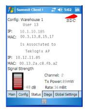
The *Status* tab provides status information including IP address and MAC address for the client radio, IP address and MAC address for the AP, signal strength, channel, transmit power and data rate.
