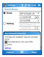
Tapping on *Connect* in the softkey bar at the bottom of the screen will automatically connect to a network that's already been set up. Tapping on *Settings* in the *network bubble* will launch the *Wireless Manager* applet.
