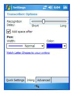
Enabling *Add space after* automatically adds a space after each word you write. The *Pen* option allows you to choose the line *Width* and *Colour*. Finally, tapping on *Match Letter Shapes to your writing* displays a screen in which you can learn how to form letters to help the hand-held to recognize the most often used characters.
