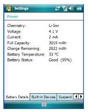
This tab lists the specifications and battery capacity status of the battery installed in the WORKABOUT PRO. This is a view-only screen.
