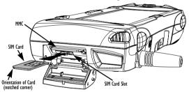
Figure 2.9 Insertion Of SIM Card
