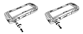
Figure 2.3 Antenna Insertion And Removal
