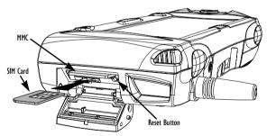
Figure 2.11 Reset Button Location
