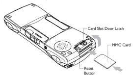
Figure 2.7 MMC Slot Location
