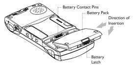
Figure 2.6 Battery Insertion
