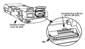
Figure 2.10 Removal Of SIM Card
