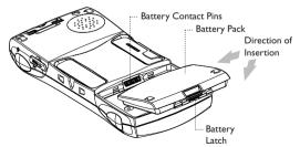
Figure 2.6 Battery Insertion
