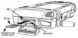
Figure 2.9 Insertion Of SIM Card
