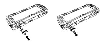
Figure 2.3 Antenna Insertion And Removal
