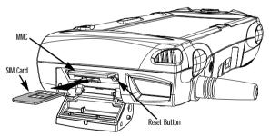
Figure 2.11 Reset Button Location
