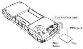
Figure 2.7 MMC Slot Location
