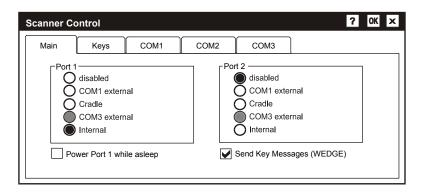
Figure 1-20 Scanner Port and Programmable Button Screen
