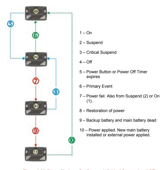
Figure 1-23 Power Modes – On, Suspend, Critical Suspend and Off
