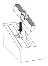
Figure 3-3 Insert Main Battery in Charge Pocket
