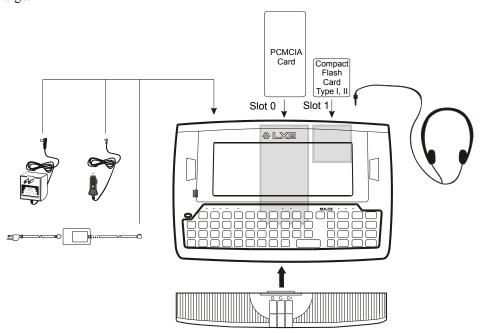
Figure 1-4 Hardware Configuration
