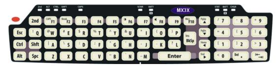
Note: The key mapping in this appendix relates to the physical keypad on the MX3X. See section titled "Input Panel" for the on-screen keypad.
