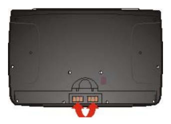
Figure 6 MX3X Battery Contacts
