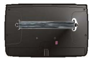
Figure 11 MX3X With Handstrap Installed
