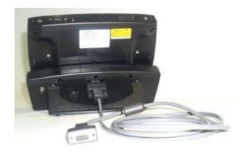
Figure 27 ActiveSync Cable Connected to Serial port on Cradle
