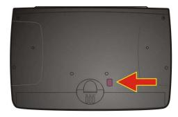
Figure 2-14 Infrared Port - COM2 Port
