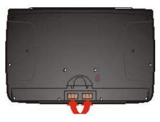
Figure 1-4 MX3X Battery Contacts
