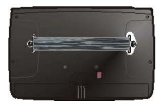
Figure 1-6 MX3X With Handstrap Installed
