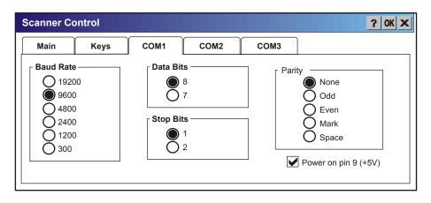
Figure 4-14 Scanner Properties / COM Port Settings
