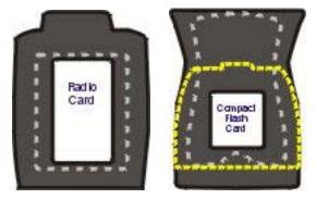
Figure 2-2 PCMCIA Radio Card and Flash Card Location
