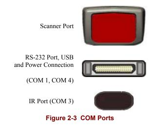
**COM 1** port is always the left RS-232 port on the base of the MX5. COM 1 port accepts RS-232, USB and AC power connectors.
