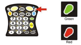
Figure 1-16 Scanner LED Location
