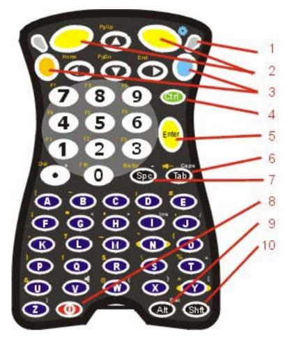
Figure 2-10 The ANSI / Batch Keypad
