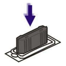
Figure 2-15 Insert Battery Pack in Charging Pocket
