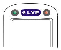
Figure 11 Scan and Decode LEDs
