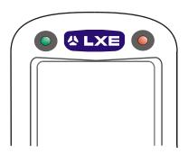
Figure 2-6 Scan and Decode LEDs
