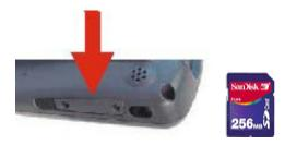
Figure 3-2 Secure Digital Memory Interface Card Location
