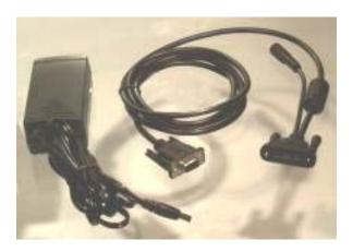
Figure 2-1 AC/DC 12V External Power Supply
