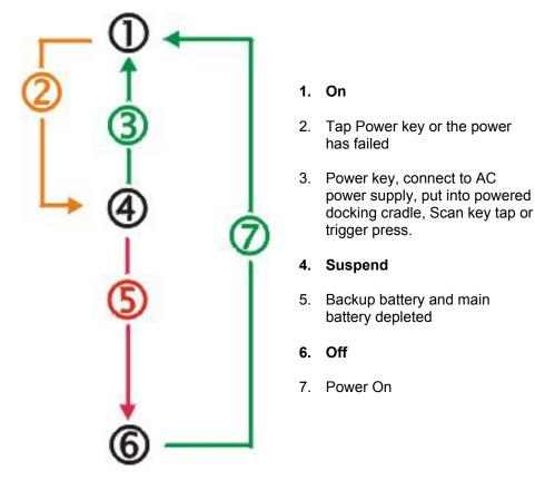
Figure 3-6 Power Modes - On, Suspend and Off
