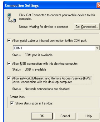
Figure 3-38 ActiveSync Connection Settings on a Windows PC
