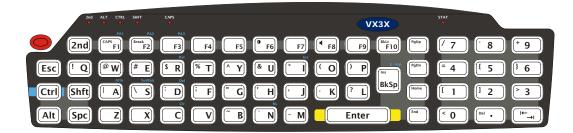
Figure A-2 IBM 3270 Specific Keypad
