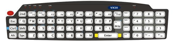
Figure 2-13 QWERTY Keyboard with IBM 3270 Overlay
