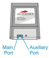
Figure 2-43 Summit Antenna Cable Connections
