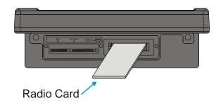
Figure 2-40 Inserting the 2.4GHz Type II PCMCIA Radio
