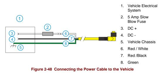
*Note:* Correct electrical polarity is required for safe and proper installation. Connecting the cable to the VX7 with the polarity reversed will cause the VX7's fuse to be blown. See the following table for wire color-coding specifics.
