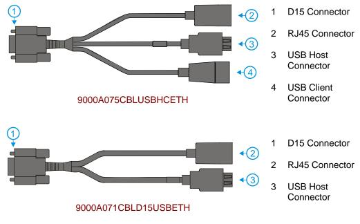
Figure 2-14 VX7 Ethernet/USB Dongle Cables
